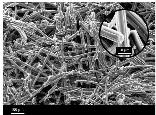
Fig. 2. Random orientation of uncoated fibers in felts (SEM, SE).
